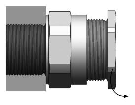
5. Pass the cable through the gland to the desired position, then tighten the seal nut using a spanner until resistance is felt (when the seal contacts the cable). Tighten with a spanner one further turn.
